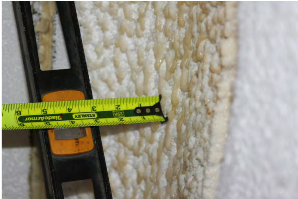
Figure 8. Right Wall: Post-Test View without Metal Sheeting. Nominal 2 3/4-in. Melting Depth at Crib Corner.
